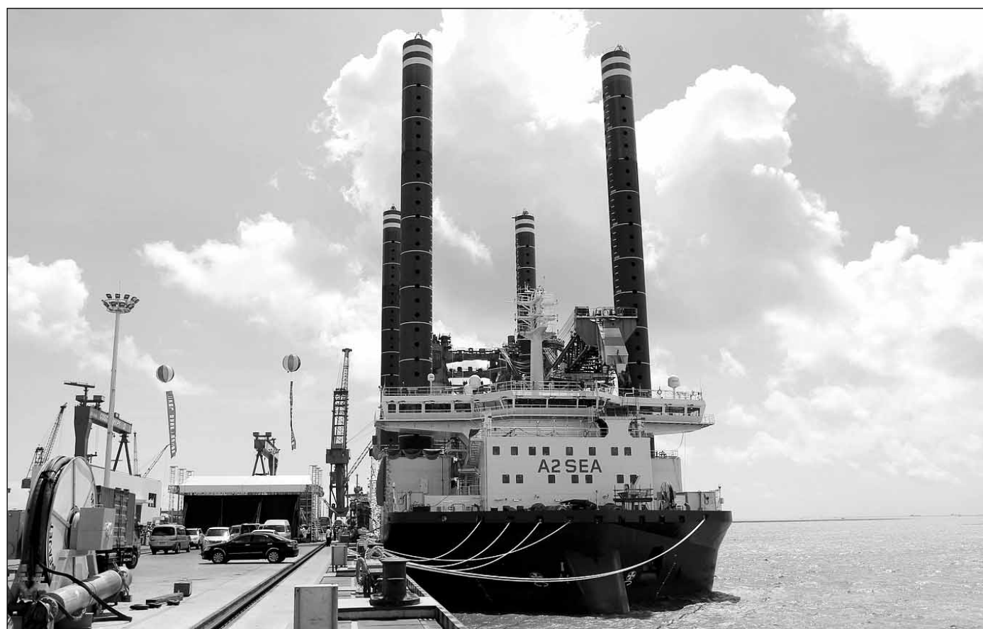
A third-generation jack-up offshore wind power installation ship in Nantong, Jiangsu province, on Tuesday. The ship, featuring a high level of automation, was designed and built by COSCO Shipyard Group Co Ltd for a Danish company.
