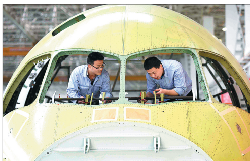
Technicians at the AVIC Chengfei Commercial Aircraft in Chengdu assemble a windshield for the nose of the C919. LIU KUN / XINHUA
